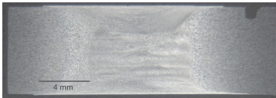
Figure 10 Transverse metallographic cross-section of a 2219 FSW made with a self-reacting tool. Note the symmetry between root and crown. The plate thickness is 8 mm. (Photo courtesy of MTS Systems Corporation, Advanced Engineering Solutions Division.)
