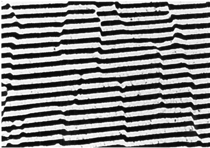
Figure 3 Lamellar microstructure of an unidirectionally solidified Al-CuAl 2 eutectic (transverse section). 1000 \times . (From Ref. 27.)
