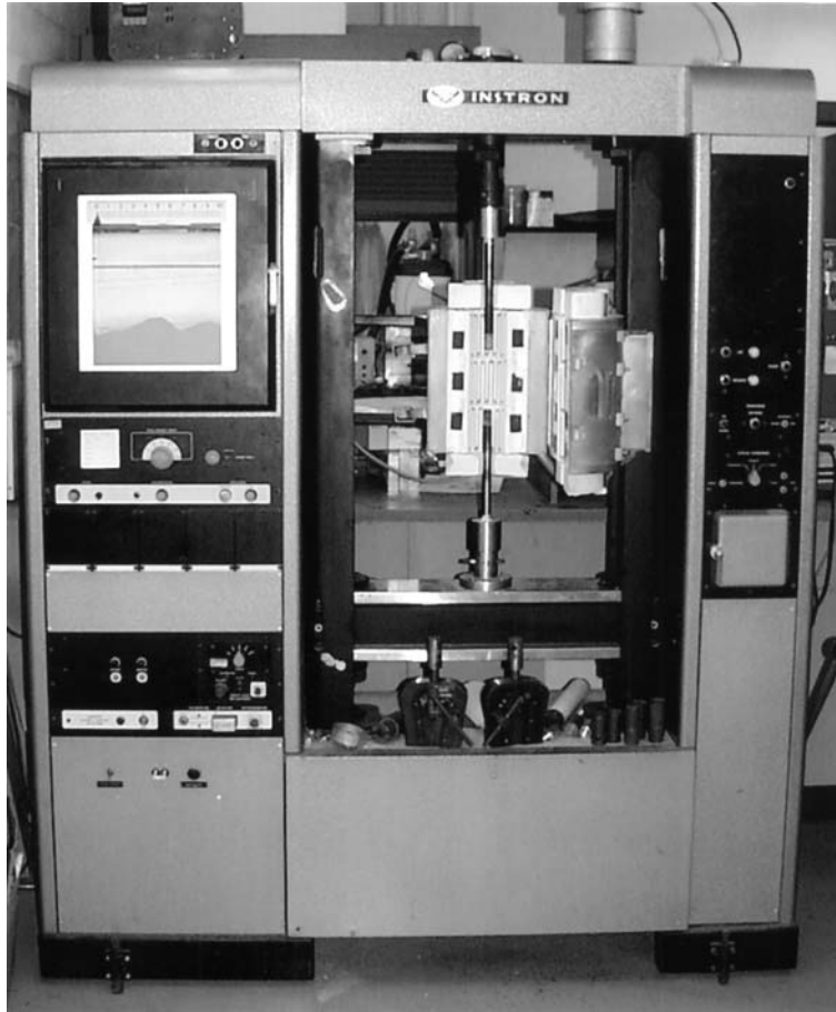
Figure 43 An example of a screw-type tensile testing machine.
