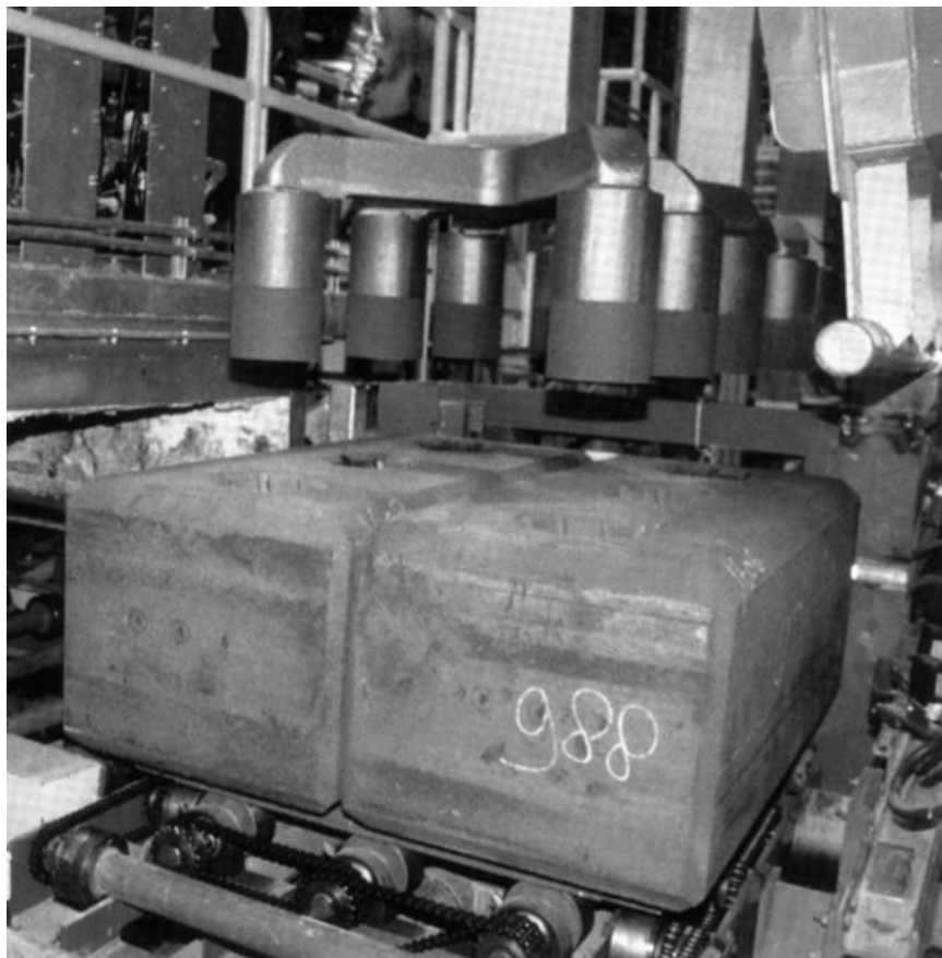
Figure 28 Rodding of anode blocks.
