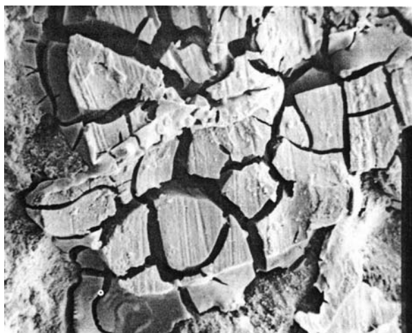
Figure 8 The surface of aluminum corroded in saltwater at room temperature has a mud crack pattern where the thick hydroxide gel dried and cracked. (From Ref. 4, with permission from ASTM.)
