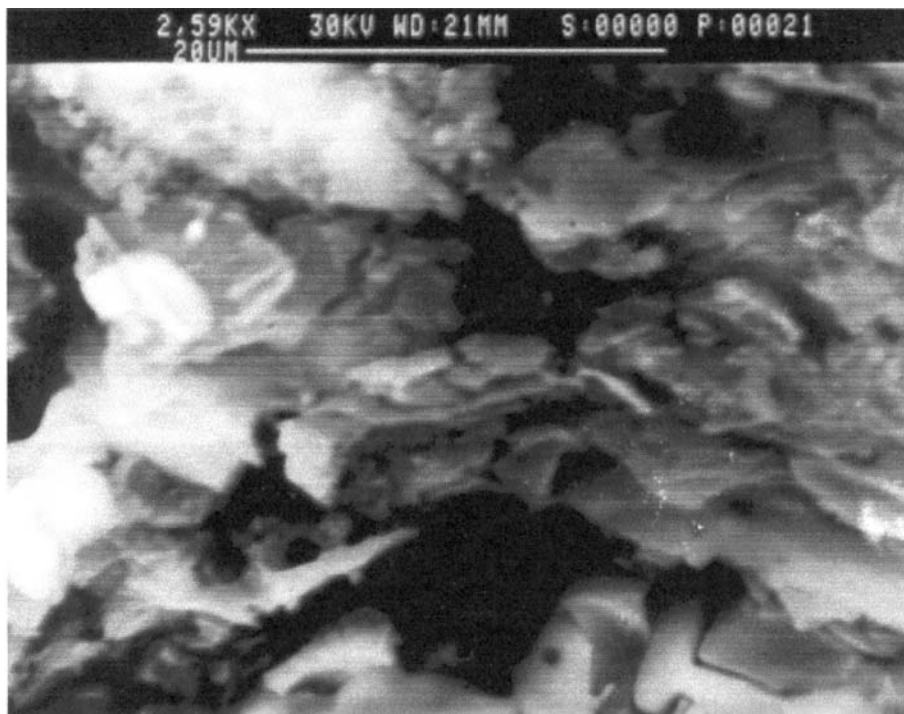
Figure 22 Back scattered image. Electron micrograph showing the oxide net fragmented after the molten salt action. (From Ref. 71.)
